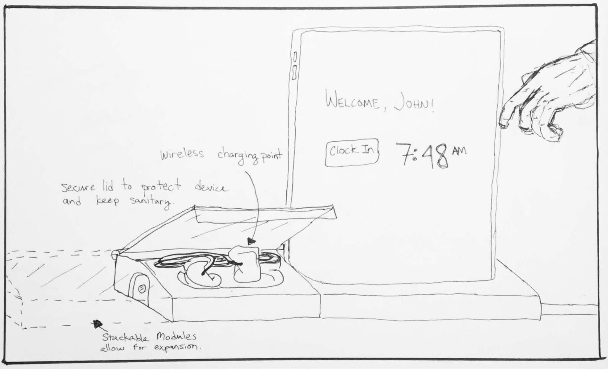
Product lives at job site. Each worker has an individual storage and charging device to keep their custom fit ear protection secure, sanitary and charged between shifts. Returning the device to its designated location removes the possibility of devices being left away from job site, thus delaying their work.
