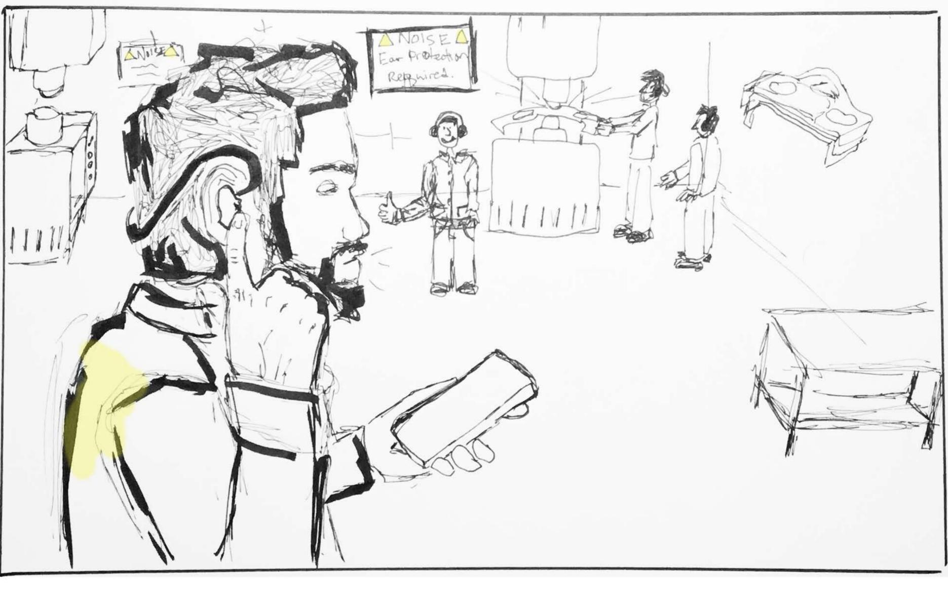
An external microphone on the hearing protection device allows workers to communicate while harmful job site noise is filtered out.
